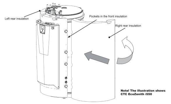
Begin with the left rear insulation. Turn out the insulation, locate it in the pockets in the front insulation and then turn it in against the tank. Repeat this procedure for the right rear insulation. Note that the right rear insulation needs to be turned out quite a lot for it to locate easily in the pockets.
