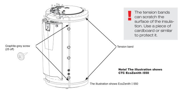
When the rear insulation is in place, tension bands can be used to hold it firmly against the tank. Attach the insulation sections to each other using the 25 graphite-grey screws provided. The screw holes are factory prepared.
