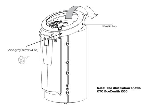
Fit the plastic top at the front and tip it backwards to locate it under the mixing valve actuator. Fit the 4 provided zinc-grey screws in the prepared holes. Ensure that the top is correctly aligned with the front.
